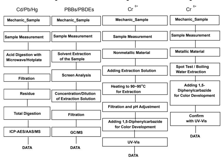
The samples were dissolved totally by pre-conditioning method according to above flow chart for Cd,Pb,Hg. Section Chief: Gilsae Yi
