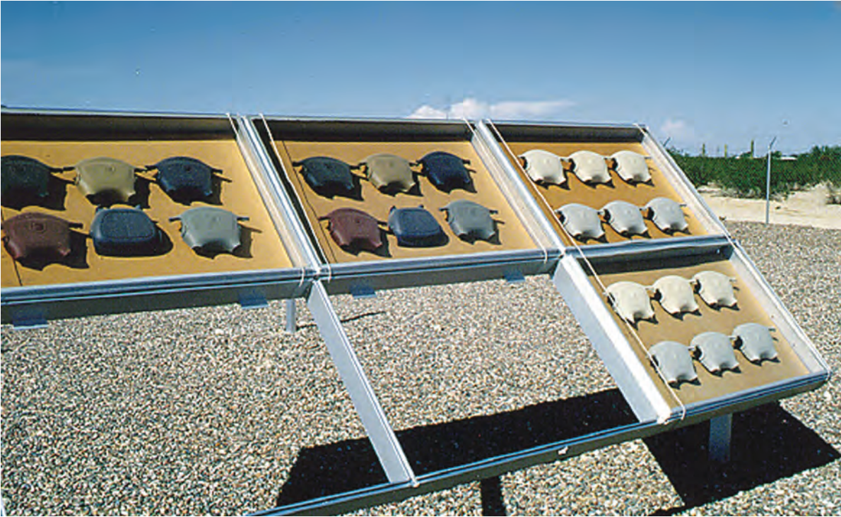
Sub-frames with window glass protect automotive interior materials tested in "under glass" exposures. These steering wheel covers are being tested at Q-Lab Arizona. ( http://www.q-lab.com/test-services/arizona.aspx )
