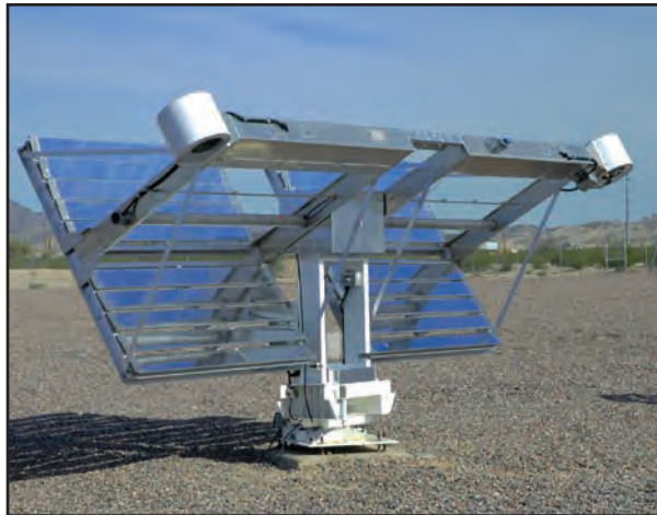
The new Q-Trac II has double the specimen capacity of the original Q-Trac.
