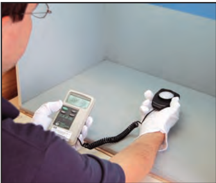
Checking correct illumination with a lux meter before a visual evaluation.
